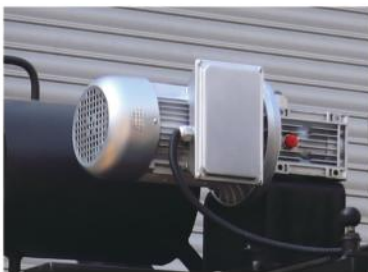
Stirring Is Driven By Motor, Speed Up Melting
