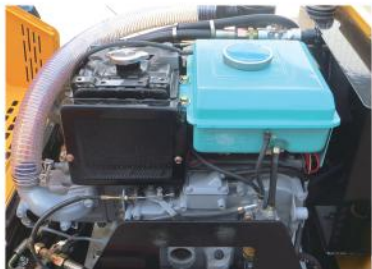
Water-Cooled Diesel Engine
