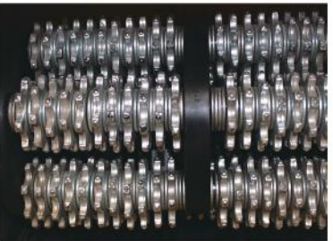
Staggered Knife Hub Design Make Sure No Milling Dead Ends
